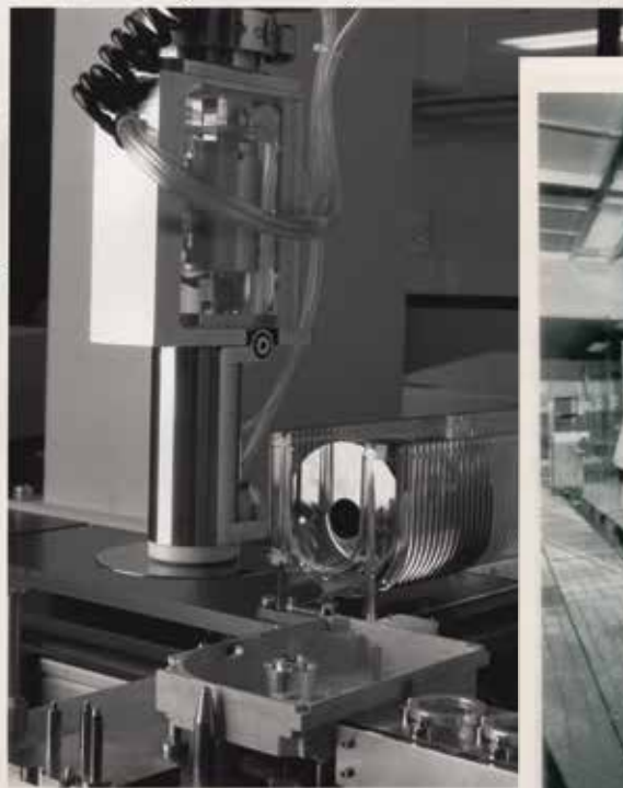
A disk loading station in Quantum's highly mechanized manufacturing facility in Milpitas, California. This plant is one of the high-capacity products in Quantum's ProDrive Series. ®
